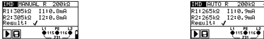
Figure 5.17: Examples of IMD test results
