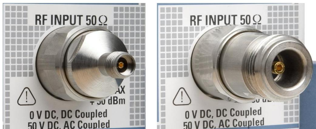
Fig. 2-2: Test instrument with Test Port Adapter Head attached.
