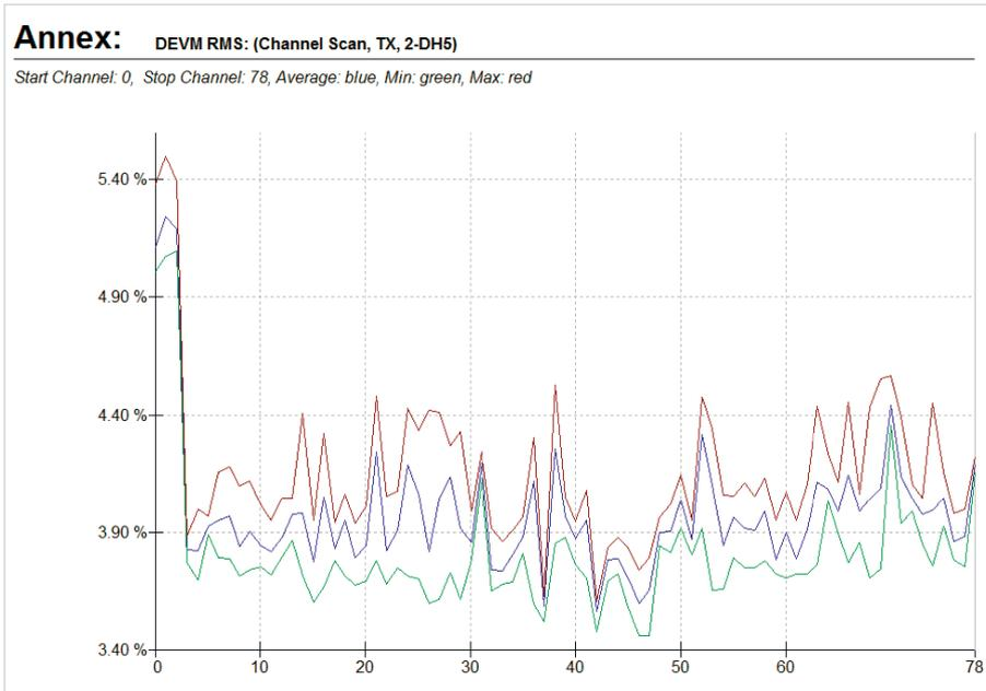
Graphic display of the measurement results delivered by R&S®CBTgo for all 79 RF channels.
