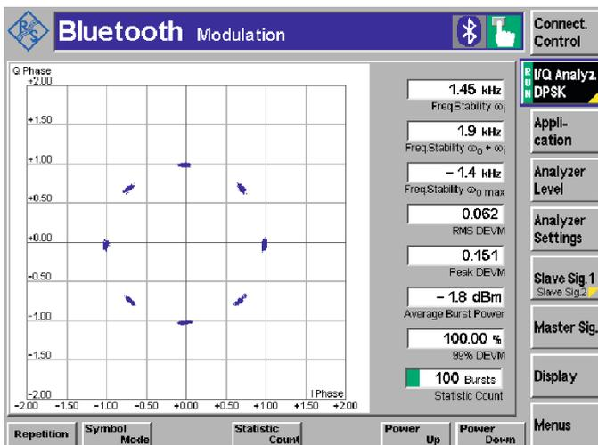
Phase difference characteristic of an EDR packet.
