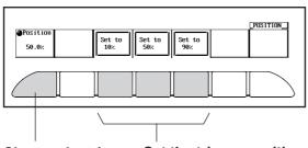
Change the trigger Set the trigger position position. (O)
