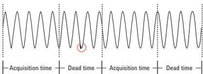
Figure 3. Reducing the dead time between acquisitions ...
