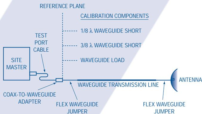
Vector Correction Avoids Bulky Waveguide Coupler
