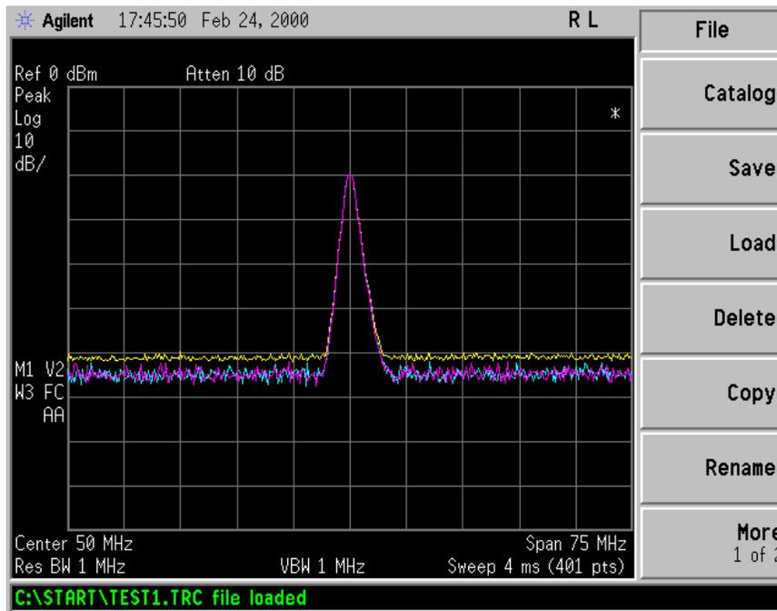
**NOTE** You should notice that the trace you saved, in this example trace 3, is loaded to trace 2. If you wish to verify this condition, remove the signal input. For Agilent E4401B and E4411B, press **Input/Output, Amptd Ref (Off)**, for all other models, press **Input/Output, Amptd Ref Out (Off)**.
