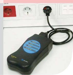
VoltScanner is a 1-phase voltage recorder for testing supply voltage on a socket in accordance with EN 50160 power quality standard.
