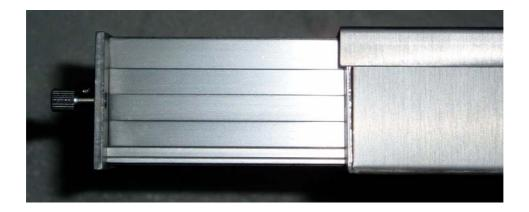
Push horizontally the module into any one of the two slots at the back of transmitter. (See the figure below for reference.) Please be careful to push the module in the right direction that the words on the panel should not be upside down, and then tighten the two screws.
