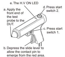
Removing the test probe from the DUT:
