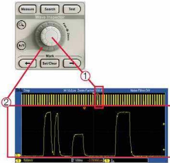
Wave Inspector controls provide unprecedented efficiency in viewing, navigating, and analyzing waveform data. Zip through your 1 M point record by turning the outer pan control (2). Get from the beginning to end in seconds. See something of interest and want to see more details? Just turn the inner zoom control (1).
