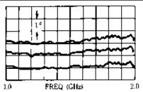
Center trace is phase response of HP 8491A -6 dB attenuator from 1.0 to 2.0 GHz taken with HP 8410 network analyzer. Top and bottom traces are  $\pm 1^{\circ}$  calibration. Linear phase component has been compensated for with a line stretcher. Response, therefore, shows nonlinear phase deviation of  $< \pm 1/2^{\circ}$  over 1 to 2 GHz band.
