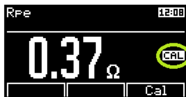
Figure 28: Incorrect compensation for the test leads
