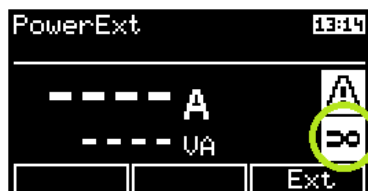
Figure 29: External input activation
