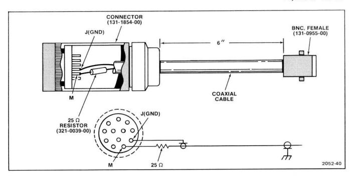
Fig. 3-1. Construction details for Special Adapter.
