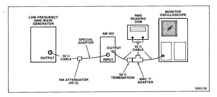
Fig. 2-1. Test setup for AC Dynamic Range Check.
