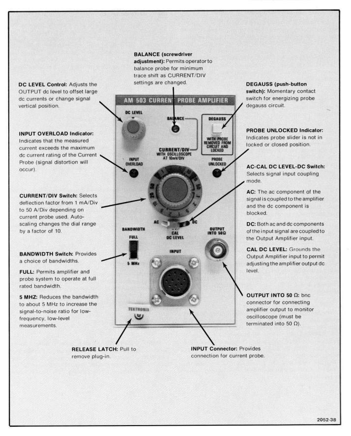
Fig. 1-2. AM 503 controls and connectors.
