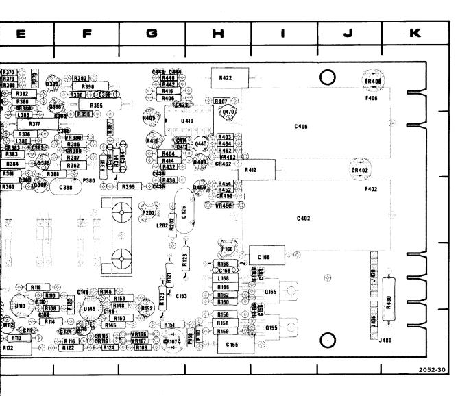
implifier circuit board with component locations of components (SN B030829 & below),
