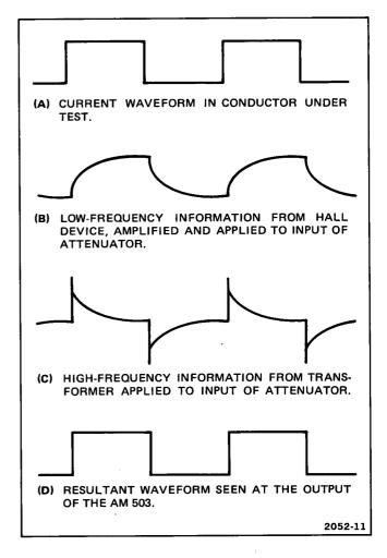
Fig. 5-1. AM 503 and probe waveforms.
