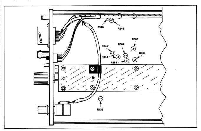
Fig. 3-3. Gain and compensation adjustment locations.
