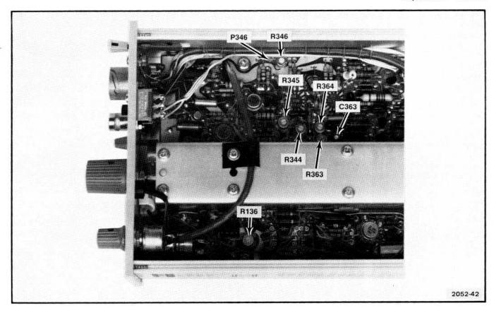
Fig. 3-3. Gain and compensation adjustment locations.
