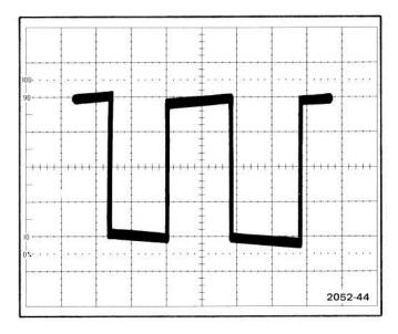
Fig. 3-4. Example of correct compensation.
