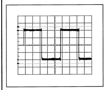
Fig. 3-4. Example of correct compensation.
