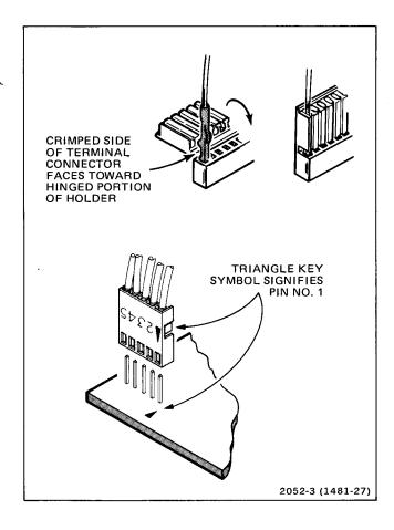
Fig. 4-3. Installation of lead-end connectors.
