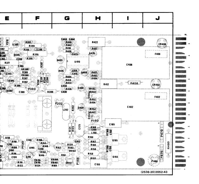
board with component locations of components (SN B030830 & above).
