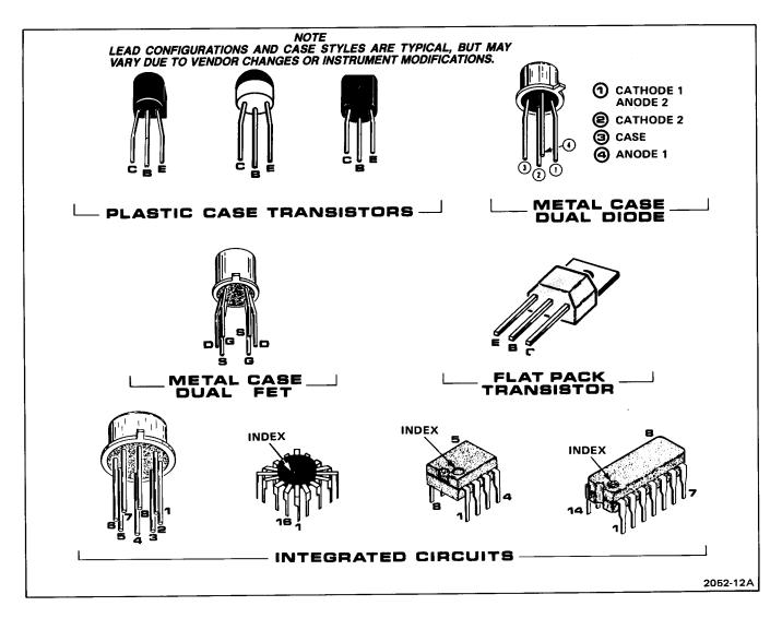
Fig. 4-2. Semiconductor lead configurations.
