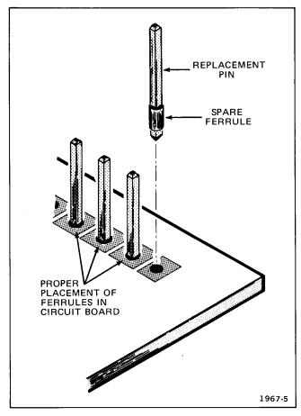
Fig. 4-4. Circuit-board pin and ferrule assembly.
