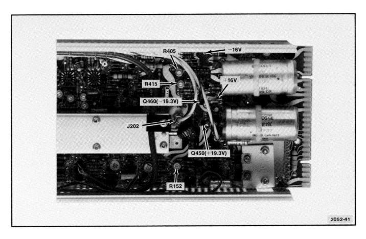
Fig. 3-2. Power supply test point and adjustment locations.
