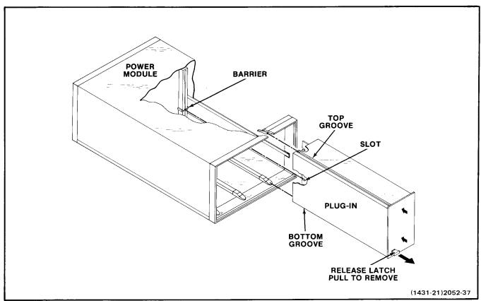
Fig. 1-1. Plug-in installation and removal.
