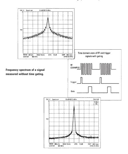
You can use time gating to accurately characterize burst-modulated signals used in data storage, television, and video equipment. Narrow gating (4395A: 6 ms min. 4396B: 2 ms min.) is ideal for testing disk drives.
