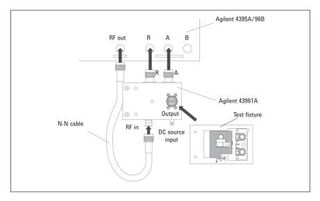
Connecting the Agilent 43961A to the Agilent 4395A/96B
