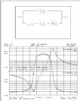
Equivalent component analysis (resonator)
