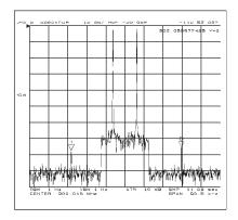
IMD measurement using list sweep function
