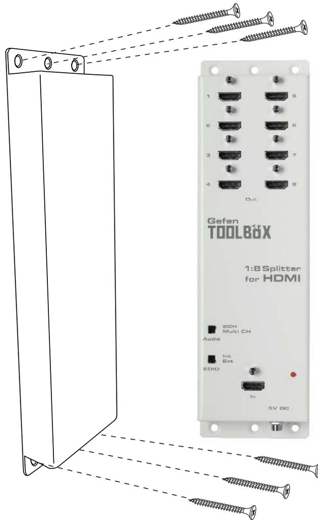
The GefenToolBox 1:8 Splitter for HDMI should be mounted vertically in a wall or cabinet with wood/drywall screws as shown in the diagram above. There should be an inch or two of clearance between the edges of the unit and any walls or vertical surfaces to allow for enough clearance for insertion and retraction of cables at the HDMI connectors.
